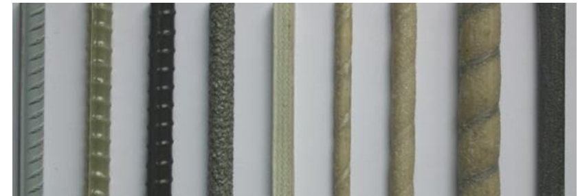
Glass or carbon rebars, with vinylester matrix, high-adherence or sandblasted surface
